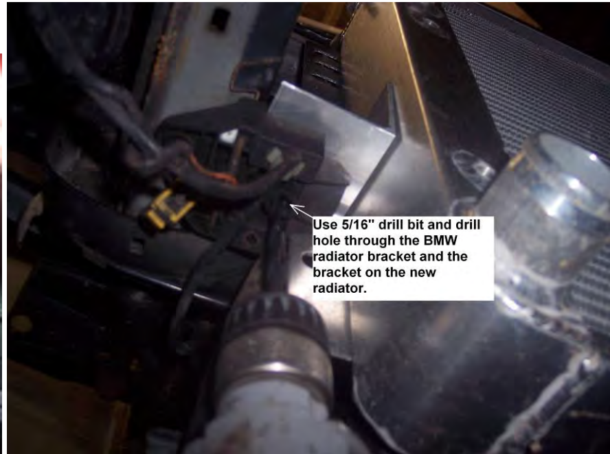
Radiator Bracket Attachment - Lower.JPG
